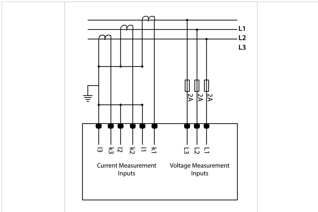
Fig. 2-5 DNTP 3 Phase Delta Connection Diagram
