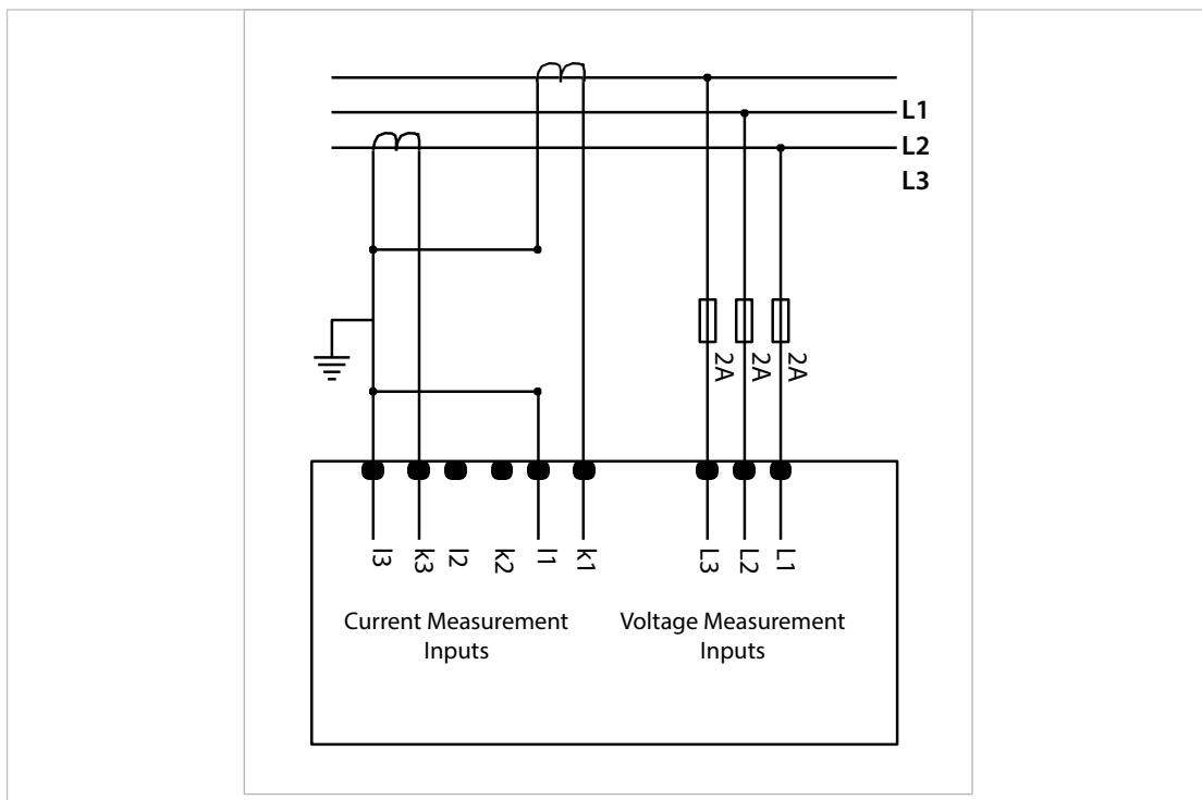
Fig. 2-6 DNTP Aron Connection Diagram
