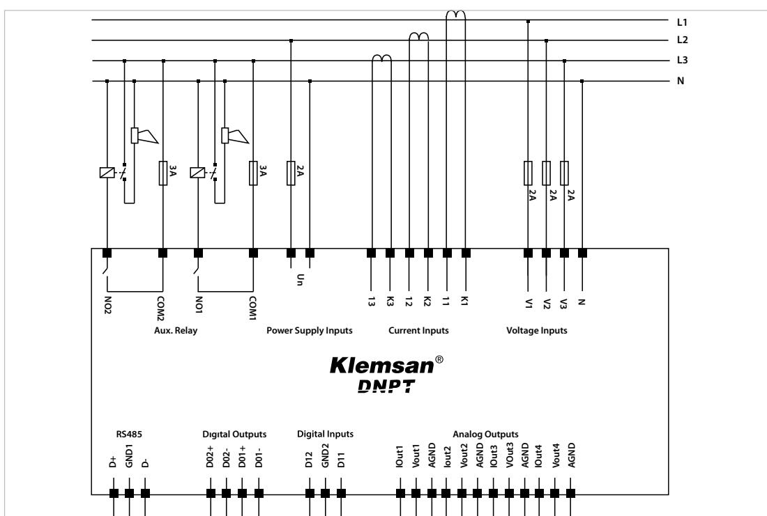
Fig. 2-4 DNPT Star (WYE) Connection Diagram
