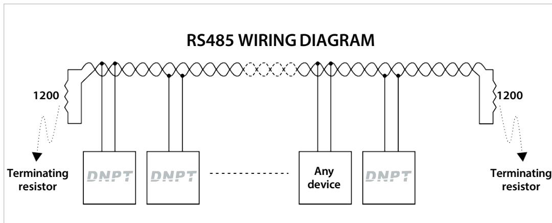
Figure 6-1 RS485 Wiring Diagram
