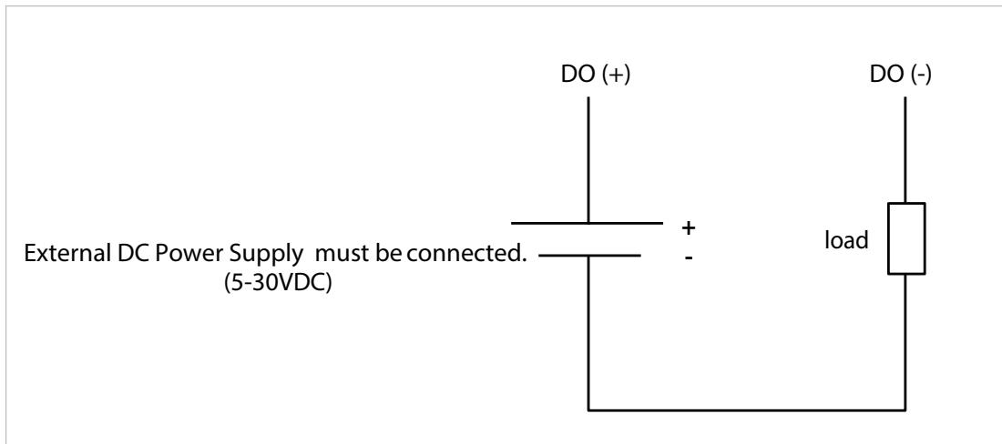
Fig. 2-7 Digital Output Connection Diagram
