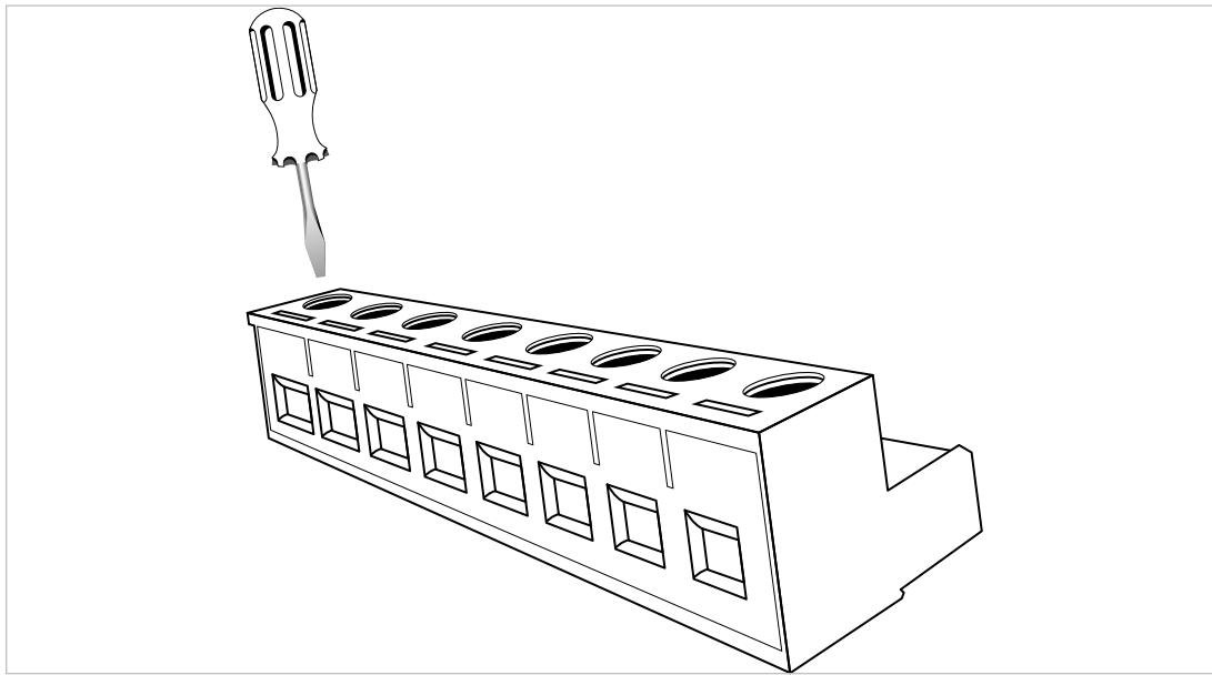
Fig. 2-1 Loosening of Terminal Block Screws
