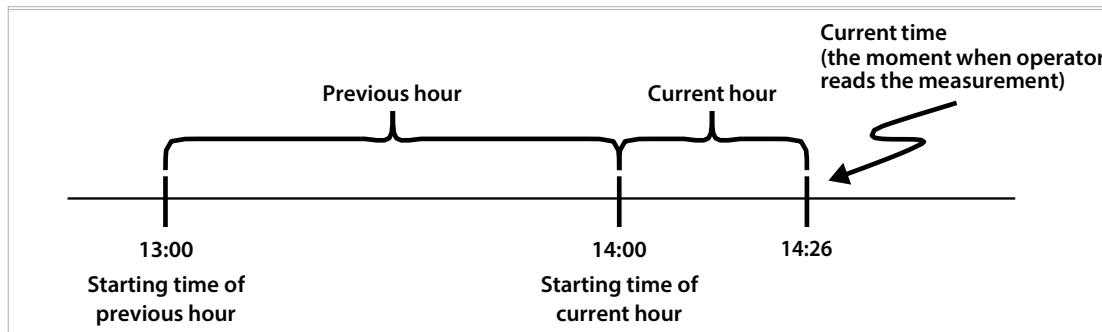
Figure 5-1 Example for Start of Hour
