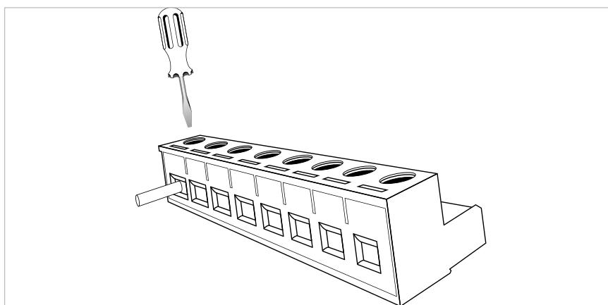
Fig. 2-3 Fixing the Cable to the Terminal Block
