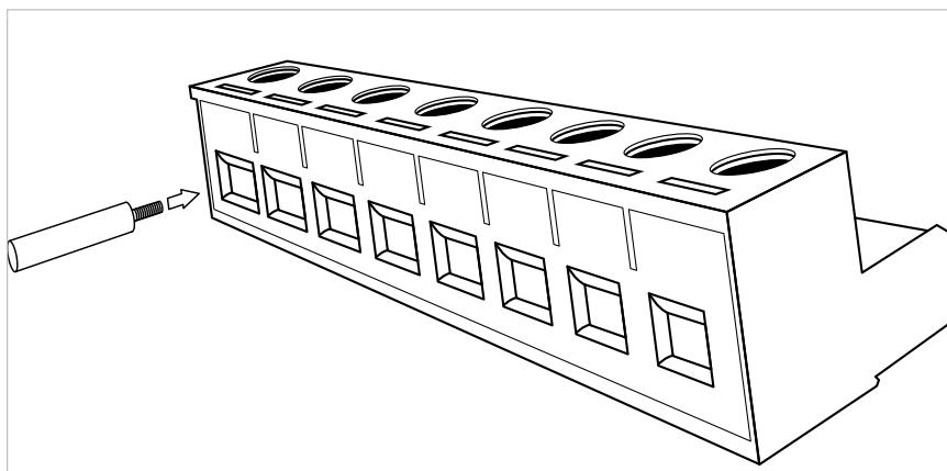
Fig. 2-2 Inserting Cable into the Terminal Block
