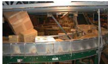
Detection of overcurrent when conveyor is jammed.
